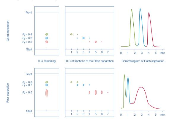
In flash chromatography, retention is expressed in column volumes (CV) which is the volume of solvent required to elute a non-retained compound or to keep it simpler, the dead volume. To isocratically elute the compound of interest 1/R<sub>f</sub> CV are required.
